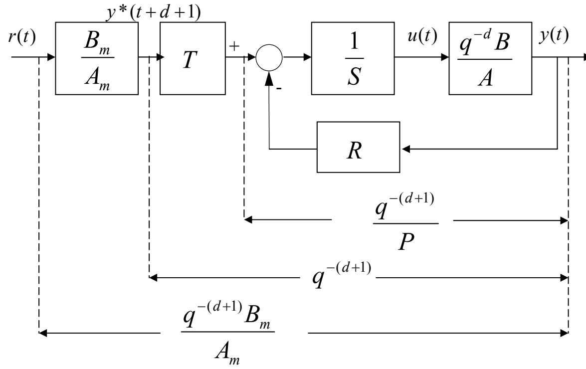
Reference signal (tracking):  $y^*(t+d+1) = \frac{B_m(q^{-1})}{A_m(q^{-1})} r(t)$
